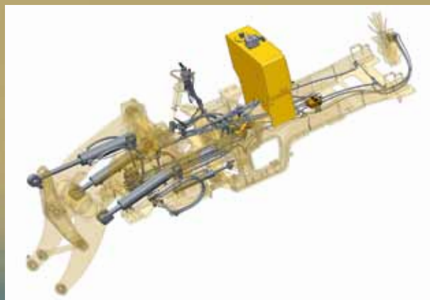
The hydraulic system components include a hydraulic reservoir with a sight gauge, a spin-on filter and suction strainers behind the operator's cab, a Load Sensing system multi-piston axial pump, a joystick controlled hydraulic control valve, boom and bucket hydraulic cylinders, a ground driven steering pump, a fan drive pump and motor, pipes and hoses.
